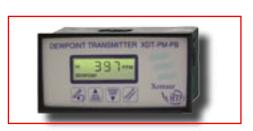
Model XDT-PM houses the transmitter in a panel mount industry standard DIN 43700 box, 7.5cm deep. Connections are made through a pluggable screw terminal block.
